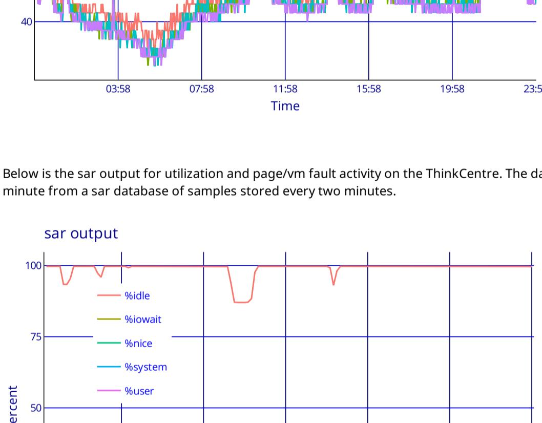
Below is the sar output for utilization and page/vm fault activity on the ThinkCentre. The data is taken every other minute from a sar database of samples stored every two minutes.
