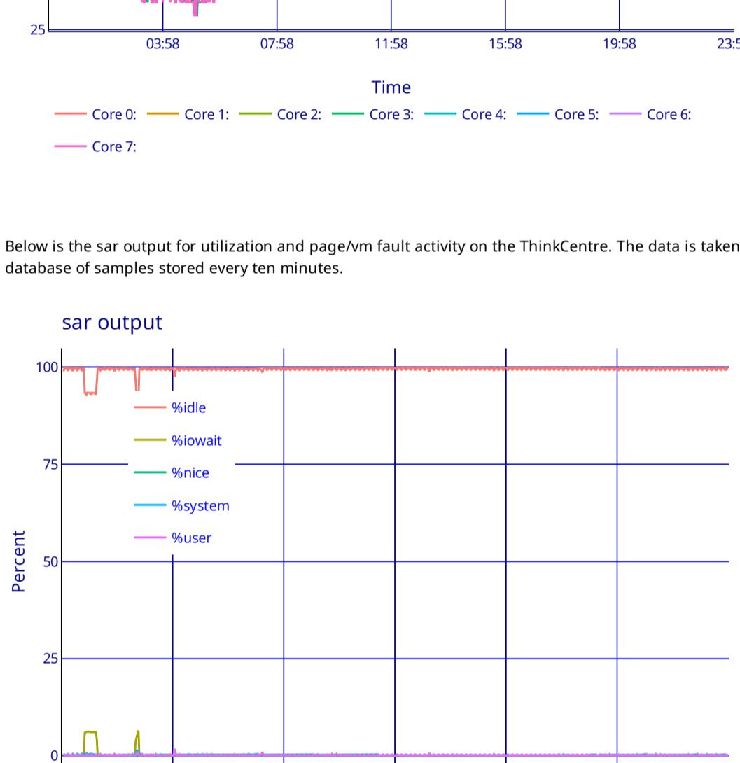
Below is the sar output for utilization and page/vm fault activity on the ThinkCentre. The data is taken every other minute from a sar database of samples stored every ten minutes.
